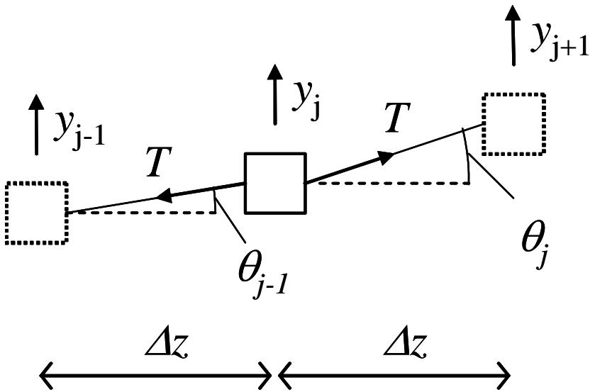
Think of the masses as the amount of mass per unit length in the  $z$  direction, that is the linear mass density  $\rho$  times  $\Delta z$ , i.e.,  $m = \rho\Delta z$
