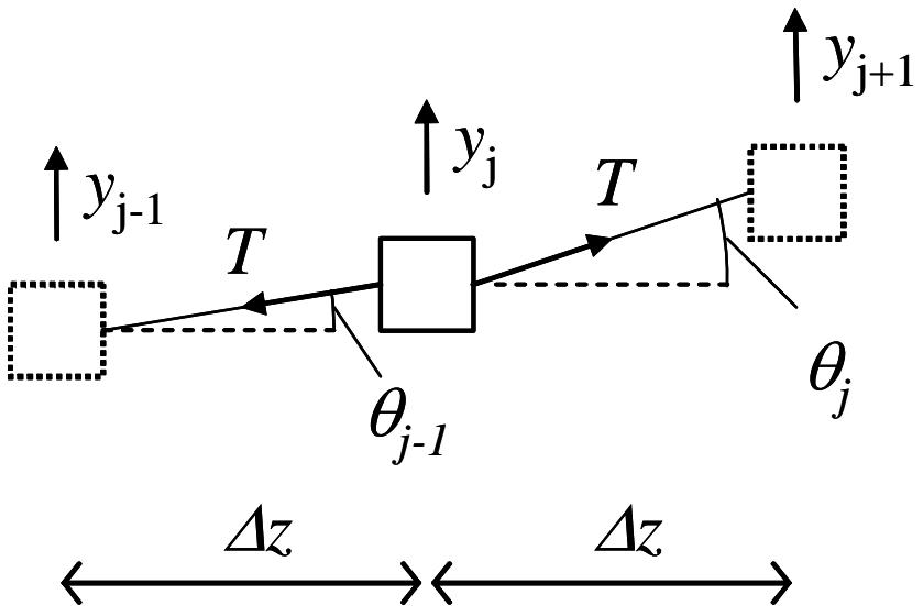
Imagine a set of identical masses connected by a string that is under a tension  $T$
