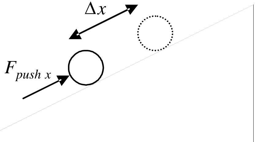
by exerting a force  $F_{pushx}$  in the  $x$  direction up the slope through a distance  $\Delta x$
