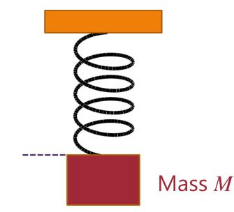
A simple spring will have a restoring force *F* acting on the mass *M* proportional to the amount *y* by which it is stretched
