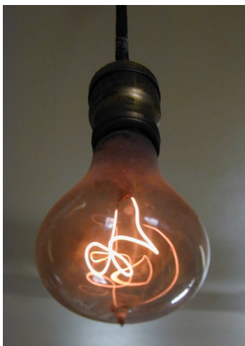
Fig. 3.2. A carbon filament light bulb at the Fire Station in Livermore, California, where it has been running essentially continuously since 1901.
